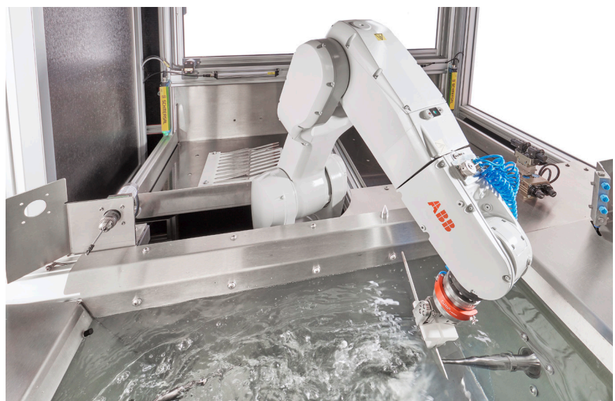
//////// Deburring of different materials Process-safe, fully automated and selective
